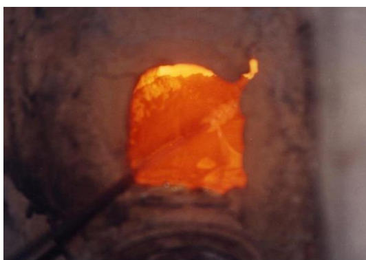
Fig.4. A furnace wound bead is being built up – North India
